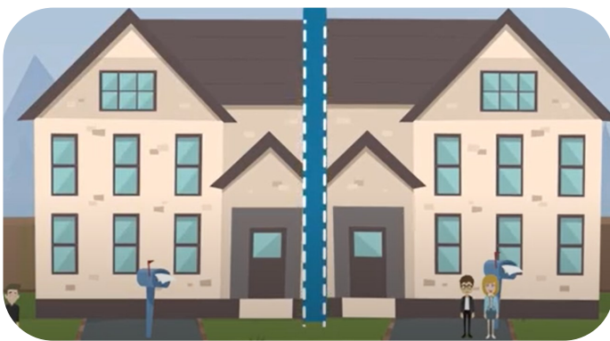
A party wall is a dividing partition between two adjacent buildings that is shared by the residents of each property.
